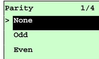
This option is used to set the RS-232 parity. The default setting is "None". Press **UP** ⬆ and **DOWN** ⬇ buttons to select the different parity and press **SELECT** button to set the value into printer. When you enter this list, the parity in the right side of ">" is the printer current setting. Press **MENU** key to cancel the setting and return to the previous menu.
