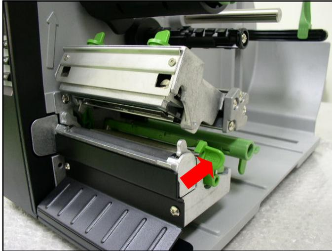
3. Install the ribbon onto the ribbon supply spindle.
