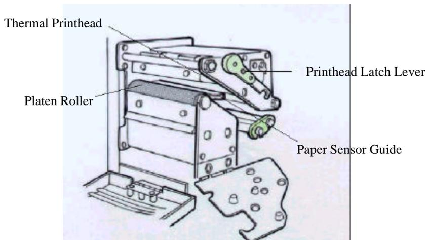
Figure 9 – **Printhead Mechanism**
