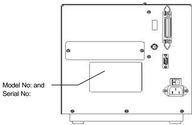
**Figure 2 - Model and Serial Number Location**
