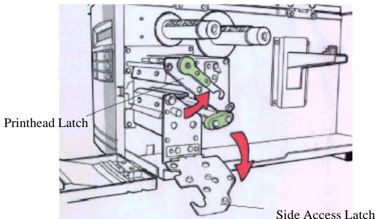
**Figure 17 - Printhead Latch and Side Access Cover**
