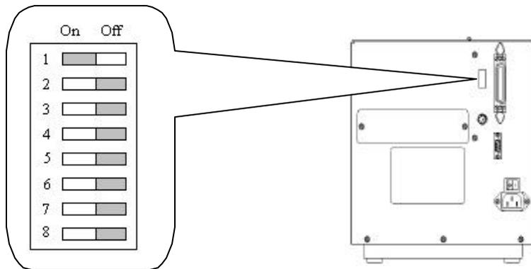
Any change in switch position is not registered until Power is cycled.
