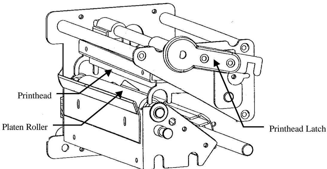
**Figure 27 - Printhead (TPH) Maintenance**
