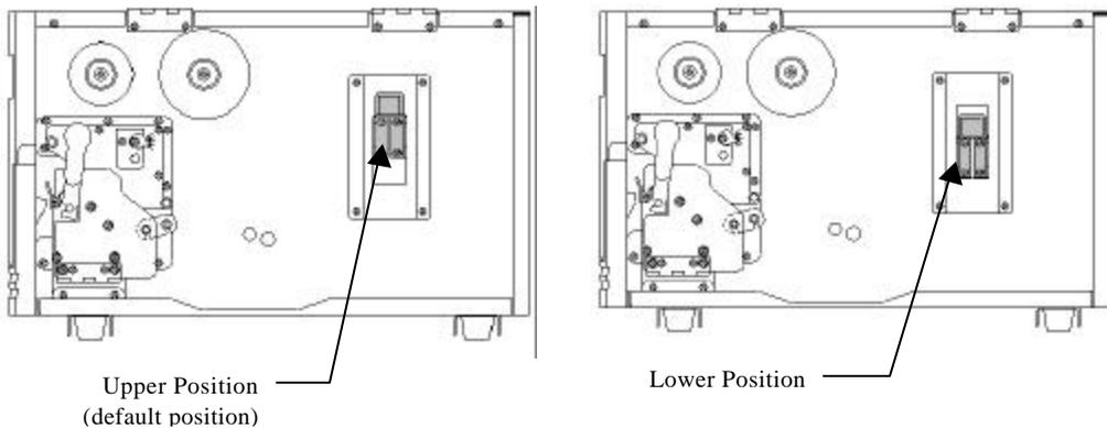
**Figure 22 - Media Supply Spindle Location**
