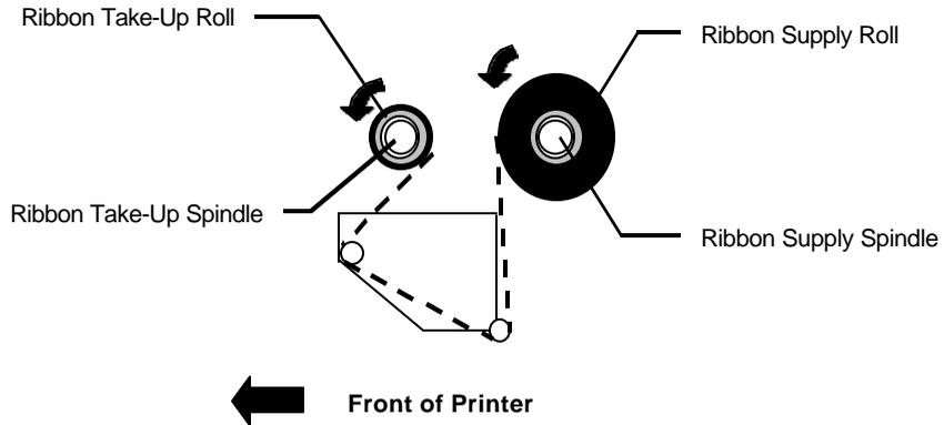
**Figure 15 - Ribbon Routing**
