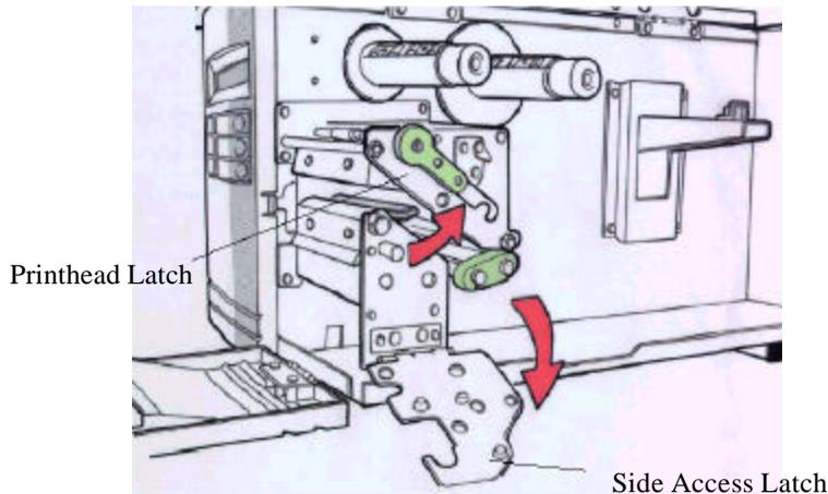
**Figure 11 - Printhead Latch and Side Access Cover**
