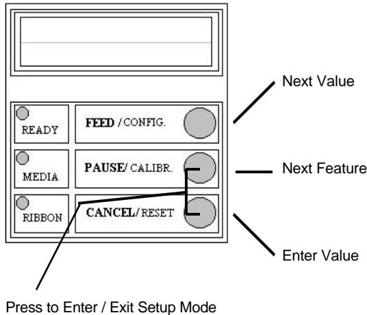
**Figure 25 - Entering into Set-up Mode**
