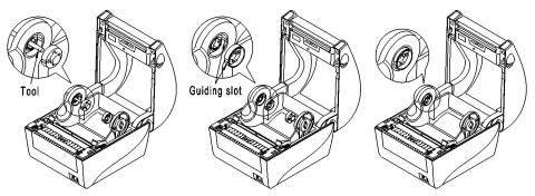
Figure 2.2-4 change the installation way of paper holder baffle
