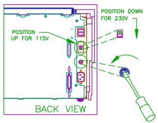
3. Make certain the fuse and fuse carrier supplied in this kit are correct for the voltage you have selected.
