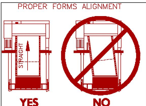
12. Verify that left form edge is in line with alignment mark.
