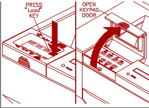
15. Load form by pressing "**Load**" key.
